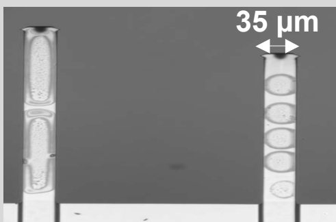
Drops as small as 35 \mu\text{m} can be placed on individual cantilevers
