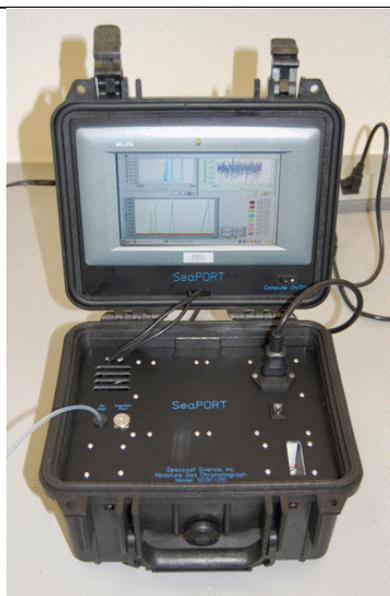
**Figure 2a.** (above). Closed Mini-GC with cell phone. **Figure 2b.** (right). Mini GC with integrated touch screen computer.
