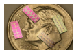
Picture of chemicapacitor sensor array on a dime. (IDT and fixed plate) are displayed. Chip size is \sim 2 \times 5 \text{ mm}
